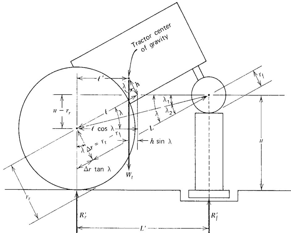
Figure7: Centre of gravity of tractor
