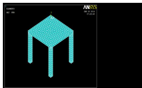
Figure1: FEA model of TABLE built in ANSYS 12.
