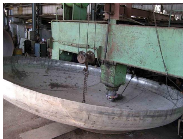
Fig 3. Bending of vessel head using a hydraulic press
