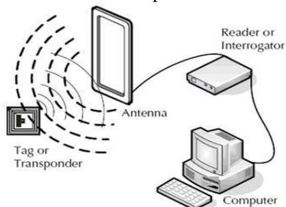
Figure 1: Radio frequency identification system
