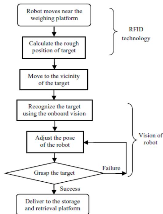
Figure 6. Flow Chart of intelligent storage and retrieval.
