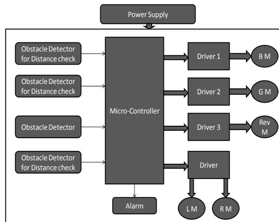
Figure 8. Control System of AGV
