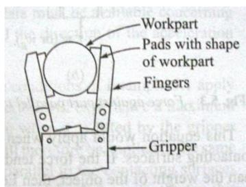
Figure 4. Single or Double type Gripper
