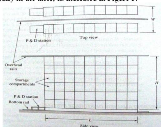
Figure 5. Sizing AS/RS Rack Structure
