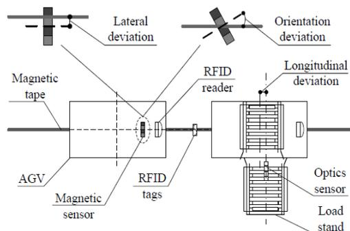
Figure 2. AGV docking process
