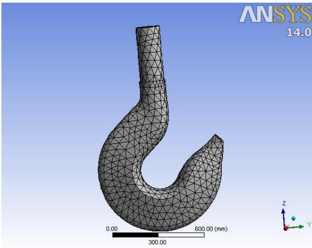
Fig. 5 Meshing of hook model
