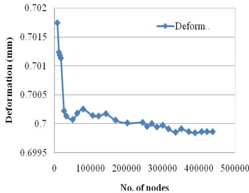
Fig. 10. Deformation convergence of hook
