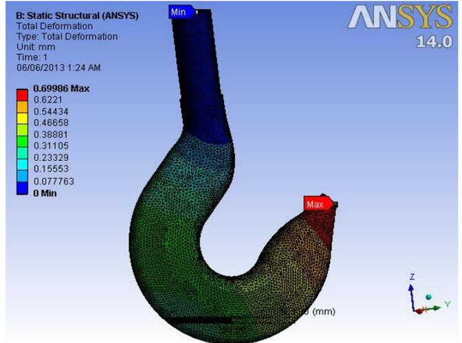
Fig. 7. Deformation analysis of hook
