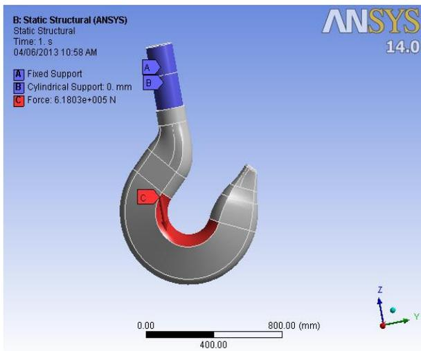
Fig. 6. Loading & boundary conditions of hook
