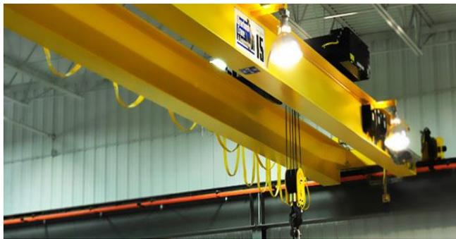
Fig. 2. Double girder overhead traveling crane
