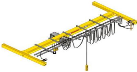
Fig. 1. Single girder overhead traveling crane
