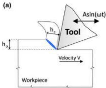
Figure 1(a): Schematic of machining with superimposed modulation a velocity modulation.  $V$  is the mean cutting velocity.  $h_o$  is the undeforms chip thickness.  $A$  is amplitude[9].
