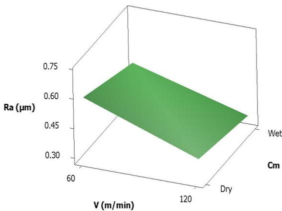
Figure 1. Effects of cutting parameters on the surface roughness.
