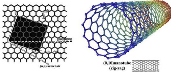
**Figure 1** As you can see in the image, there is armchair and zigzag config. Represented by (n,n) for armchair & (0,10) for zig-zag
