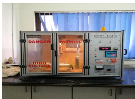
Figure 2: Actual setup of Electrospinning machine
