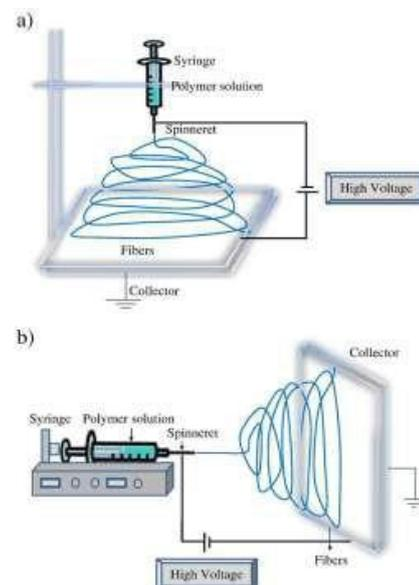
Figure 1. Schematic diagram of set up of electrospinning apparatus
