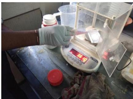
Figure 3. Actual weight measurement of nylon 6,6 and formic acid 25ml
