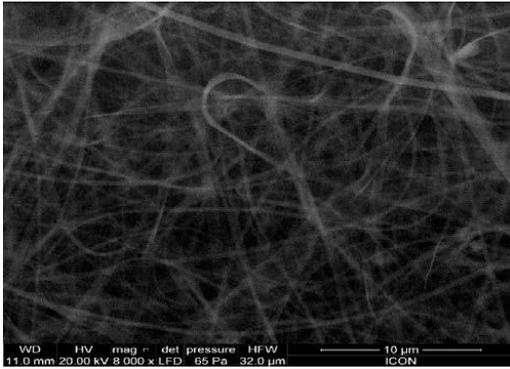
Figure 7: SEM image of Nylon 6,6
