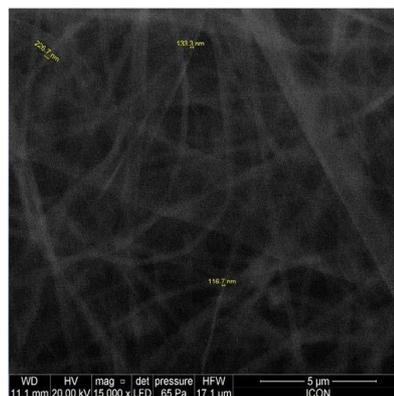
Figure 6: SEM of Nylon 6,6(116.7nm) –Distance-13cm, Voltage- 22kV Flow rate-0.4ml/hr.
