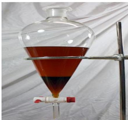
Figure 3: Separating funnel for layer separation
