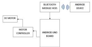
Figure 1: Block Diagram of Voice control elevator
