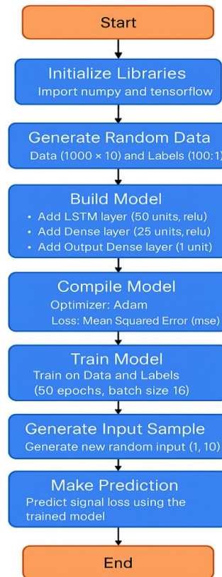
Figure 4 : the flowchart illustrating the machine learning pipeline for training a neural network to predict signal loss.
