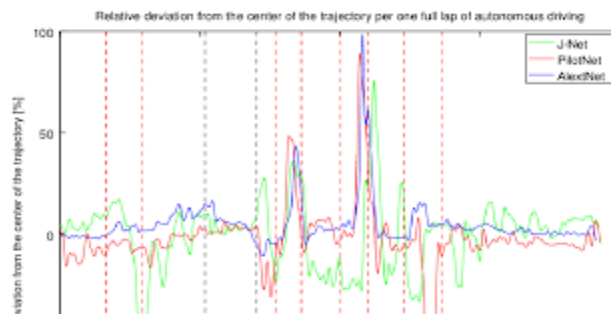
Figure 11: Percentage of a lap driven autonomously that deviates from the centered trajectory.
