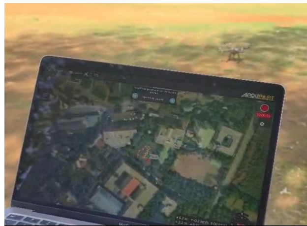
Figure 6. Waypoint-based autonomous flight mission planning for rescue response system using ground control software
