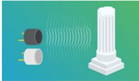
Fig -2: Ultrasonic Time-of-Flight Measurement
