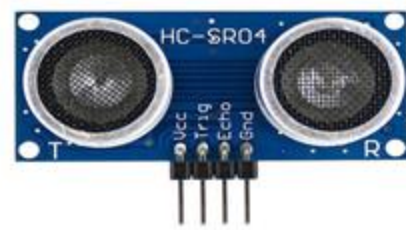
Fig -3: Ultrasonic Transmitter & Receiver
