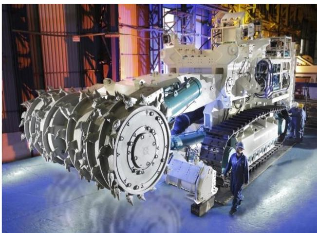
Figure 1. Underwater ROV models developed by Royal IHC, Netherland for deep sea mining.[7]
